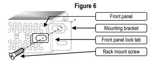
To close: Slide the lock tab toward the left over the front panel and tighten the screw.Note: When loosening the rack mount screw, it may be necessary to support the rear of the unit.
